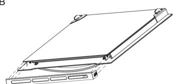
c. The inner glass pulled out from beneath plastic fixed block. After cleaning, the inner glass insert the following plastic fixed block, then install the above plastic mounting block.
