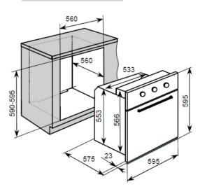
Note. It is a requirement for a ventillation gap to be cut into the oven cabinet as per the diagrams on this page.
